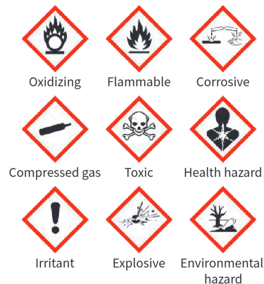
▲ Figure 3 These are the international hazard symbols and their meanings.
